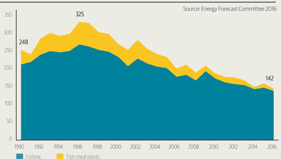
Fuel consumption by the fishing fleet is determined by the total allowable catch and pursuit of fish stocks is calculated or estimated as average consumption in litres or kilograms per unit of catch. The composition of the fleet is a major factor here, as oil consumption varies greatly depending upon the fishing gear and the type and size of vessel.
